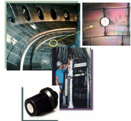
Measured erosion rate from DiMES, C \sim 4 \text{ nm/s}
